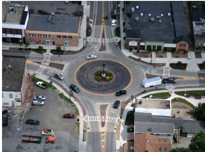
Example of a roundabout
