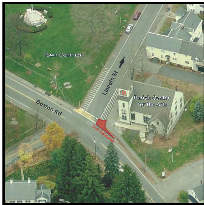
Figure 8: Conceptual design of a curb extension at the intersection of Lincoln St and Boston Rd.
