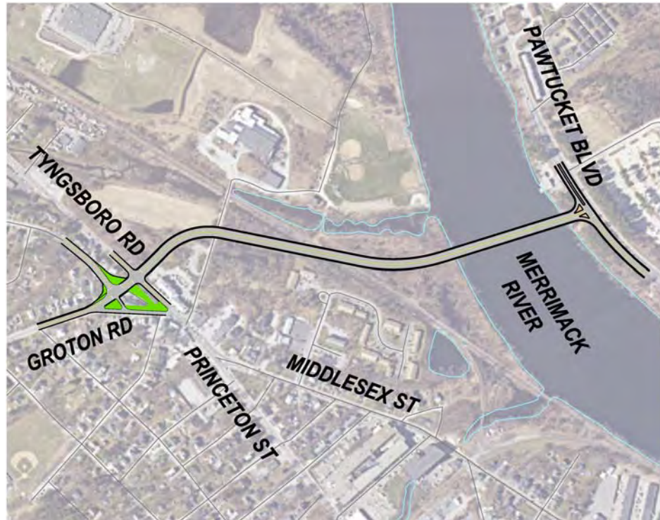
Figure 5-17 Alternative 7: Western Relocation Alignment – Vinal Square
